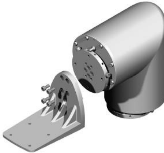
Fig. 12 Fitting the side platform
